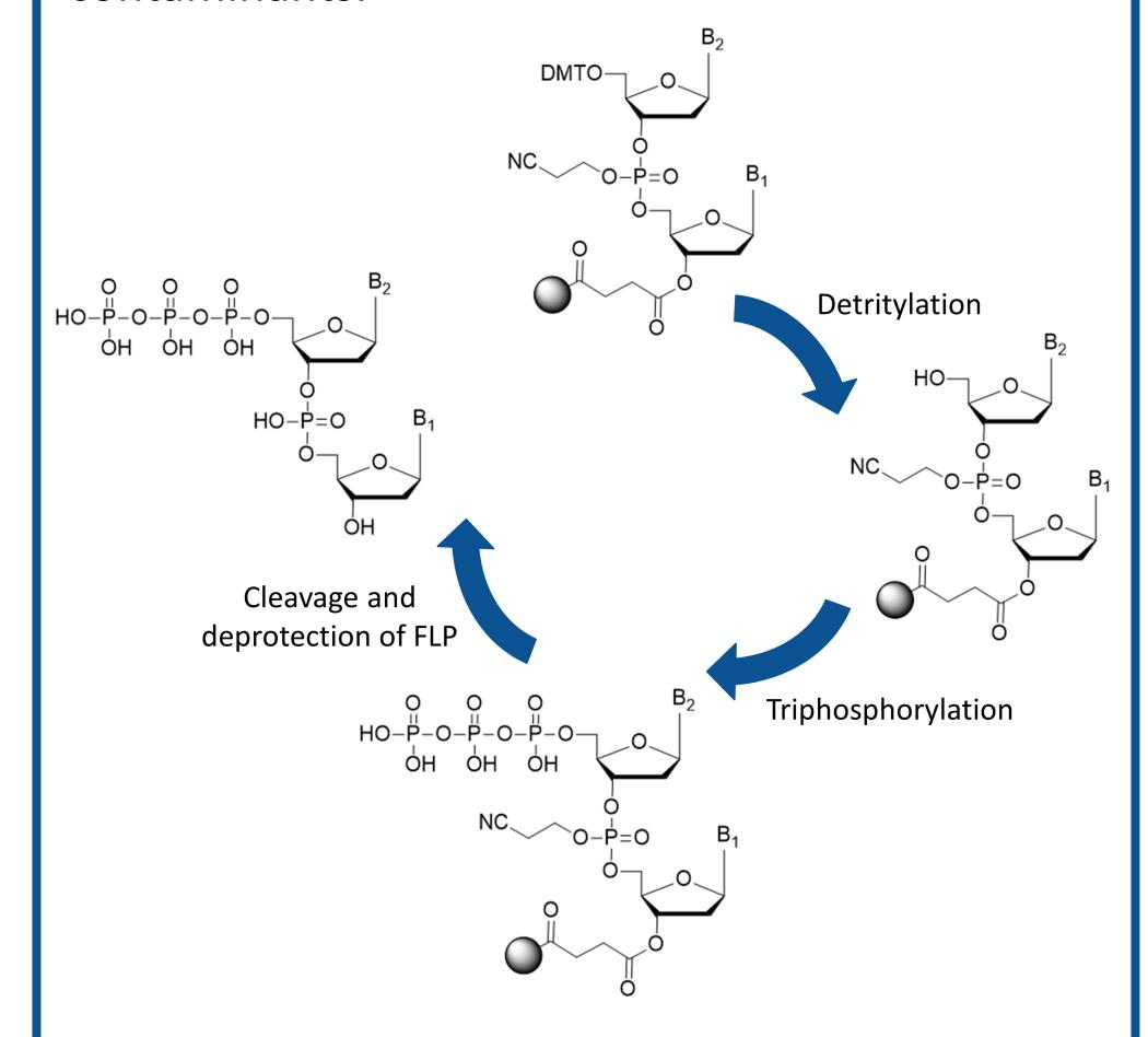
Figure 1. Triphosphorylation of oligonucleotide
